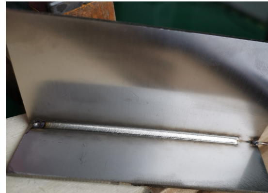
T joint welding test done
